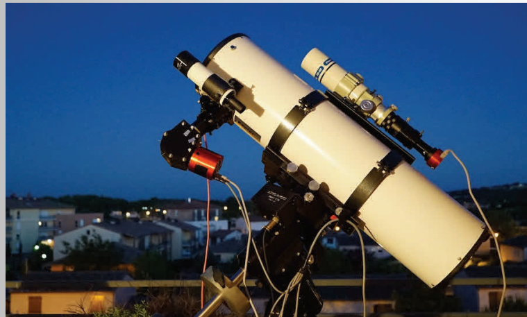
Fig. 3: The first light on a Kepler 200 mm f/5 telescope (no CMOS camera has been used but a ASI1600MM cooled model).
