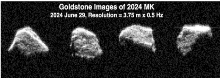
Selected delay-Doppler radar images of 2024 MK obtained on June 29 when the asteroid was at about one lunar distance and approaching Earth. Resolution is 3.75 m x 0.5 Hz. Each panel shows a weighted sum of data that span about 20 seconds. D55-14 transmitted and D55-13 received.
